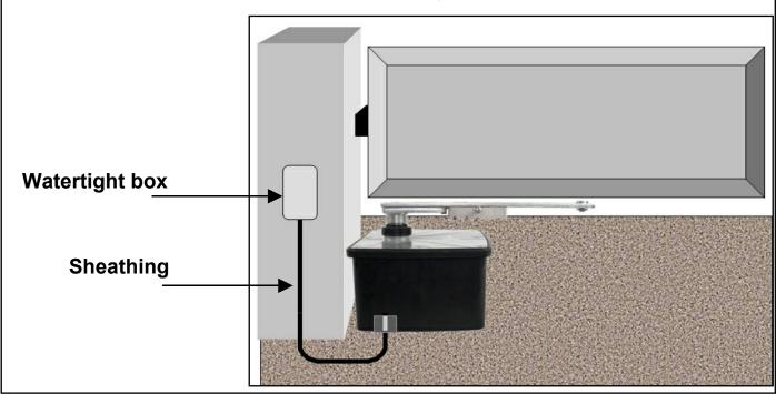
Place the operator into the hole, position and level it so that there is a distance of 85mm **(see pict.)** between ground level and the gate wing, cement firmly and wait for it to dry before assembling the levers.
